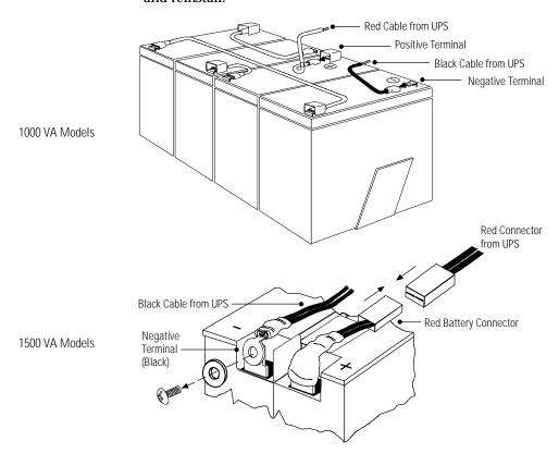
Figure 16. Internal Battery Connections
